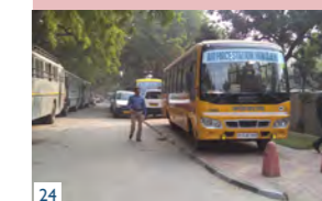
24 Absence of barriers on edges allowing encroachment
